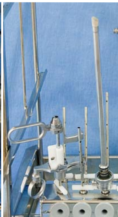
Loading example on MIS Instrument ramp. Use a spring to prevent the instrument from moving during the wash process.
