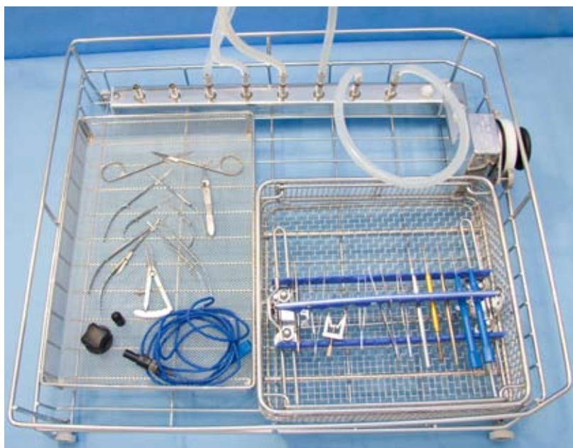
Loading example on 1345 with ophthalmic ramp. To prevent unnecessary loss of water pressure, the unused openings should be plugged with silicon hoses.
