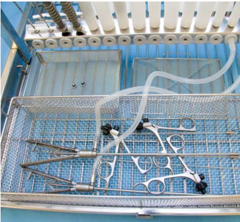
Place the fine mesh trays on the shelf. Make sure they don't stand directly under the MIS ramp to prevent cleaning shadows.
