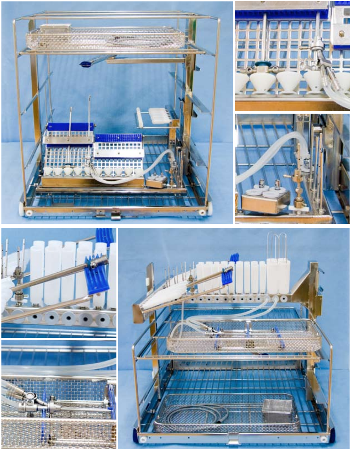
Place the albaran in the Instrument holding system and connect silicon hoses.
