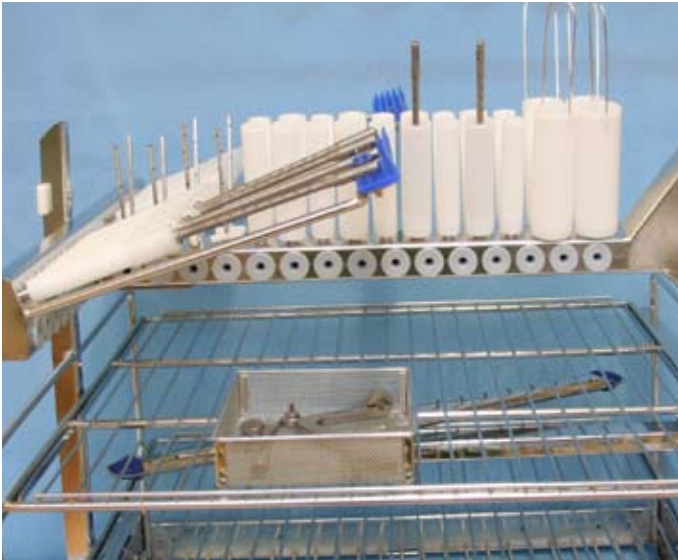
Loading example on a MIS-cart. Both used and unused instruments are placed in DIN trays on injectors. The container can either be placed on the MIS-cart or on a separate wash cart.
