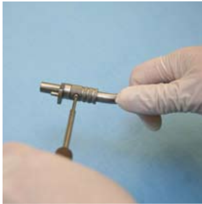
B.2 Dismantle the screw. The cup holder with block is now correctly separated.
