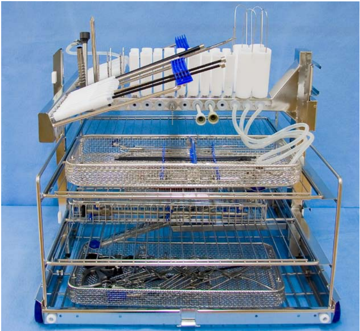
Loading example on MIS-cart. All tubular instruments are connected to injectors. Solid instruments and telescope are placed in trays.
