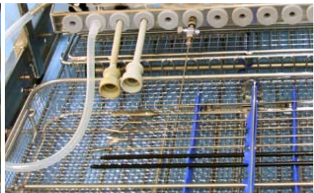
Loading example on MIS-cart. All tubular instruments are connected to injectors. Solid instruments and telescope are placed in trays.
