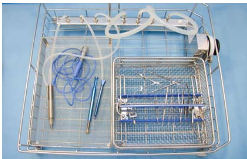
Loading example on 1345 with ophthalmic ramp. To prevent unnecessary loss of water pressure, the unused openings should be plugged with silicon hoses.
