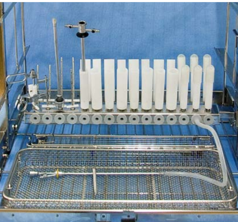
Loading example on MIS Instrument ramp. Use a spring to prevent the instrument from moving during the wash process.
