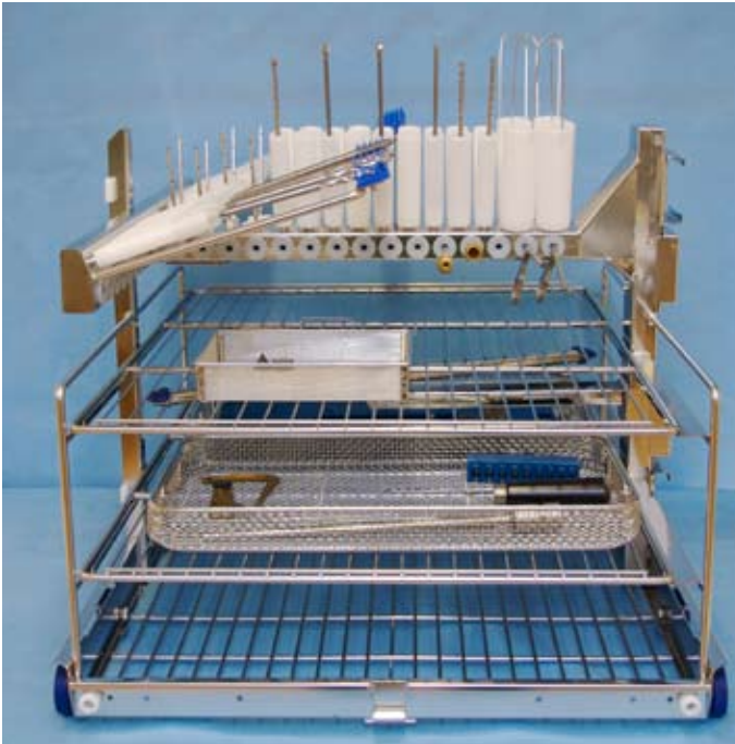
This is a loading example on MIS-cart. Place all tubular instruments in injectors and the solid instruments in DIN trays. Small parts are placed in a fine mesh tray.
