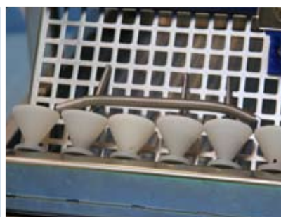
Use a spring to prevent light instruments from moving during the cleaning process. Art No. 123618 (L=100). Art No. 468525000 (L=160)
