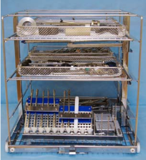
Loading example on OP-wash cart, 4 levels equipped with Rack for Tubular Instruments and Clamp Injector Head. In total there are 8 tubular instruments.
