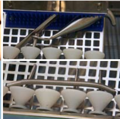
Use a spring to fix small tubular instruments.
