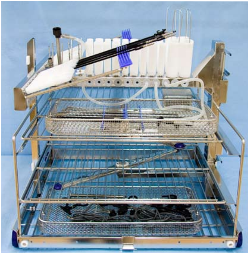
Loading example on a MIS-cart. Connect the tubular instruments to injectors and place the rod in the Instrument holding system.
